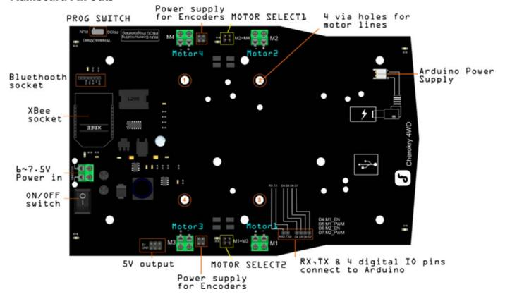
In the above diagram the 4 digital I/O pins in the lower-right corner can connect to any digital pin of an Arduino or similar microcontroller. In order for it to work you must make sure the correct pins are assigned in your code.
