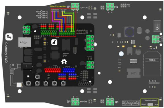
programming & Xbee Switch
