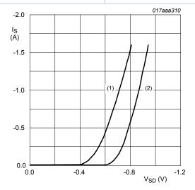
$V_{GS} = 0 V$ (1)  $T_j = 150 °C$ (2)  $T_i = 25 °C$
