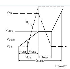
Fig. 15. Gate charge waveform definitions
