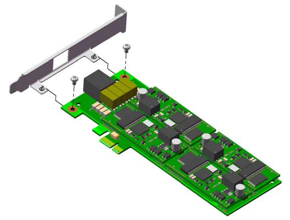
3. Mount the low profile bracket using the screws you removed in Step 1.
