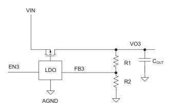
Figure 2: LDO Regulator External Feedback.
