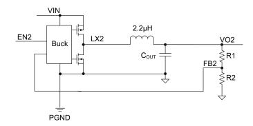
Figure 4: Buck Converter External Feedback.
