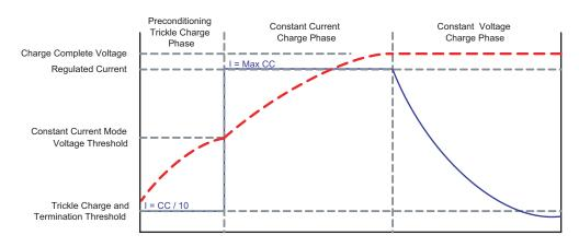
Figure 1: Current vs. Voltage Profile During Charging Phases.
