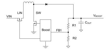
Figure 3: Boost Converter External Feedback.
