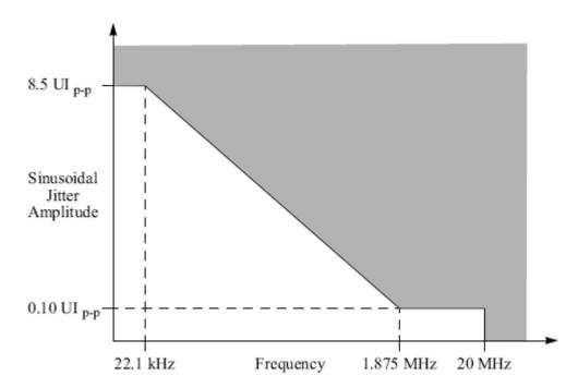
Figure 16 Single Frequency Sinusoidal Jitter Limits
