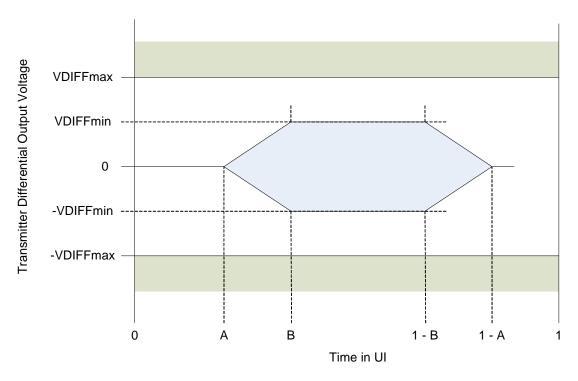
Figure 15 Transmitter Output Compliance Mask
