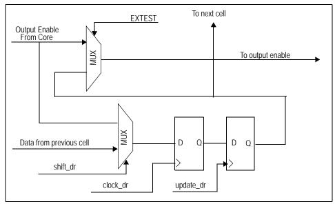
Figure 23 Diagram of Output Enable Cell
