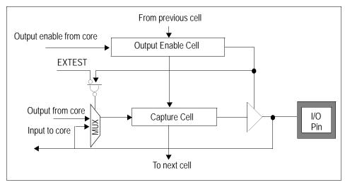
Figure 24 Diagram of Bidirectional Cell
