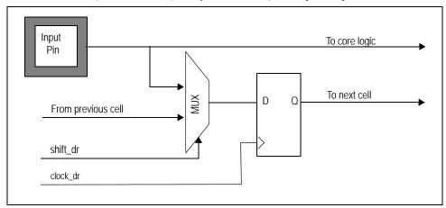
Figure 21 Diagram of Observe-only Input Cell
