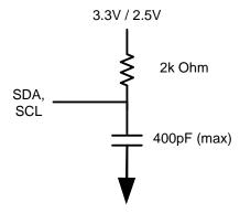
Figure 6 AC Output Test Load (I<sup>2</sup>C)
