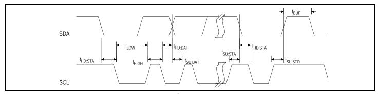
Figure 12 I<sup>2</sup>C Timing Waveforms
