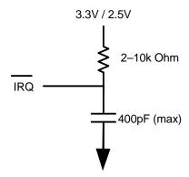
Figure 5 AC Output Test Load (IRQ)
