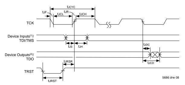
Figure 27 JTAG Timing Specifications
