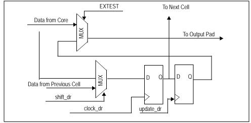
Figure 22 Diagram of Output Cell
