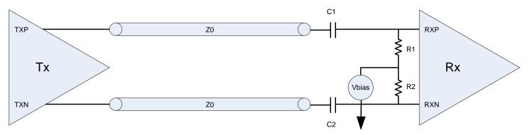
Figure 7 sRIO Lanes Test Load
