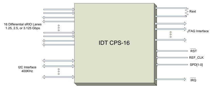
Figure 3 Diagram of the CPS-16 Interfaces
