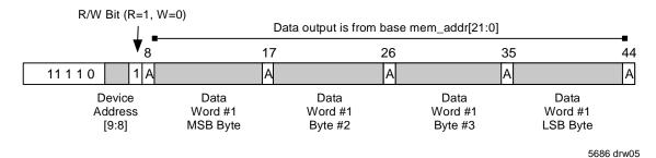
Figure 9 Read Protocol with 10-bit Slave Address (ADS=1)
