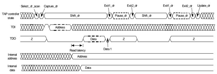
Figure 26 Implementation of read during configuration register access
