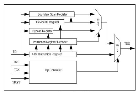
Figure 19 Diagram of the JTAG Logic
