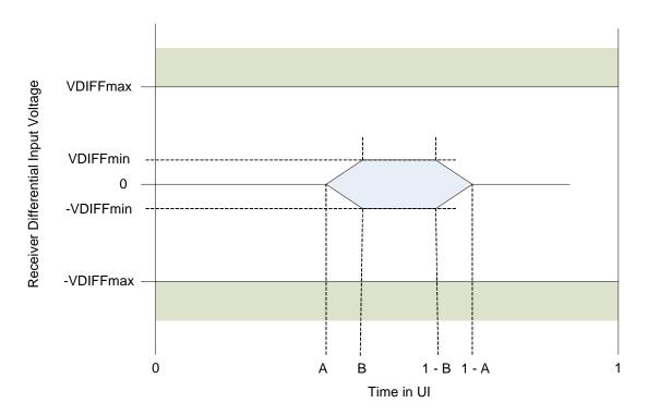
Figure 17 Receiver Input Compliance Mask
