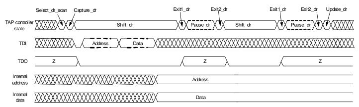
Figure 25 Implementation of write during configuration register access
