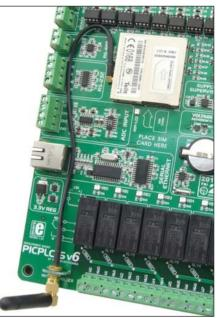
Figure 9-4: GSM module with antenna
