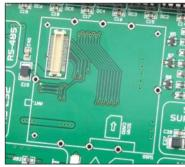
Figure 9-1: GSM connector
