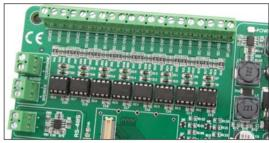
Figure 12-2: Optocouplers with relevant connectors
