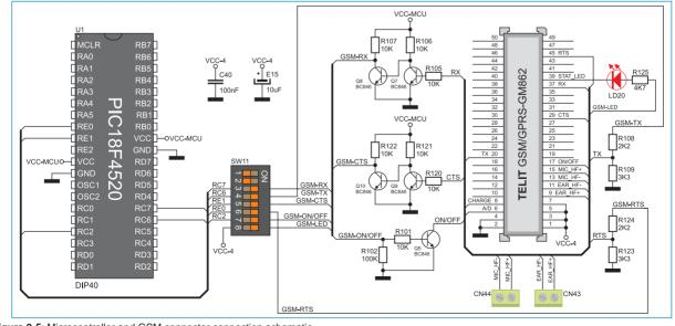
Figure 9-5: Microcontroller and GSM connector connection schematic
