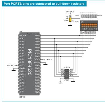
Figure 13-4: Port PORTB connection schematic
