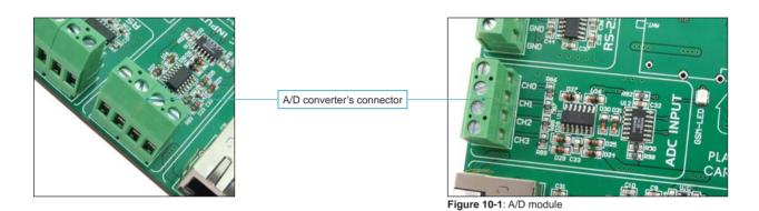
A/D converter communicates to the microcontroller using SPI communication vçc SW10 MCLF GNE MCP1541 E10 RA1 RB RA2 RB4 RA3 vçc 4.096 RA4 1144 D26 D28 厶 1N4148 SW9 -ovcc-mcu D29  $\infty$ 1N4148 1N4148  $\sim$ VCC-MCUO GND OSC<sup>7</sup> і N D24 CN1 1N4148 4 1N4148 D31 D25 1N/1/1 1N4148 R90 D88 CN1 1K VCC-MCU RC3 vçc RD0 CH2 C32 C33 RD1 100nl DIP40
