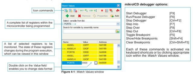
The mikroICD debugger also offers functions such as running a program step by step (single stepping), pausing the program execution to examine the state of currently active registers using breakpoints, tracking the values of some variables etc. The following example illustrates a step-by-step program execution using the *Step Over* command.
