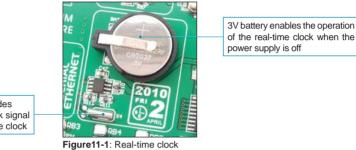
Quartz-crystal provides accuracy of the clock signal – used by the real-time clock
