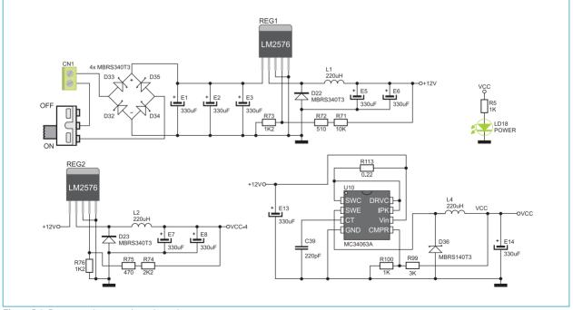
Figure 5-2: Power supply connection schematic
