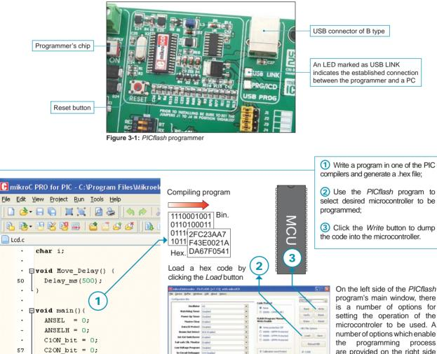
Write a code in one of the PIC compilers, generate a .hex file, and employ the on-board programmer to load the code into the microcontroller.
