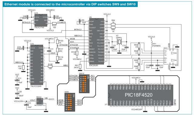
Figure 8-2: Ethernet module connection schematic
