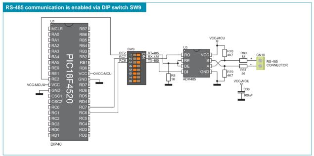
Figure 7-2: RS-485 module connection schematic
