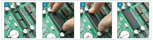
Figure 2-3: Placing microcontroller into the socket
