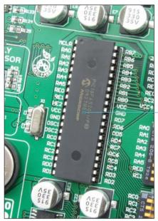
Figure 2-1: Microcontroller in DIP40 package
