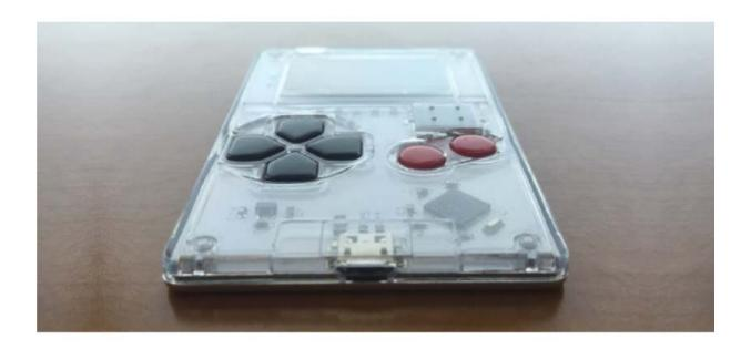
A polycarbonate front, ultra thin circuit board, and stamped metal back gave us the ultimate combination.
