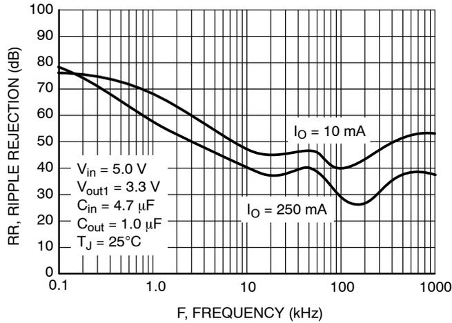
**Figure 9. Ripple Rejection vs. Frequency for V<sub>out1</sub>**
