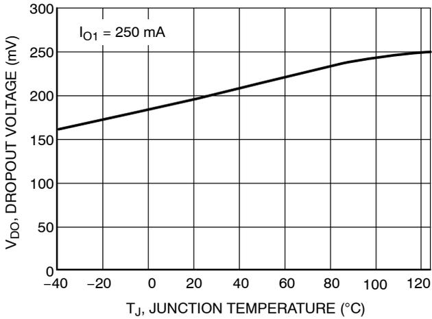
Figure 5. Dropout Voltage vs. Temperature for  $V_{out1}$
