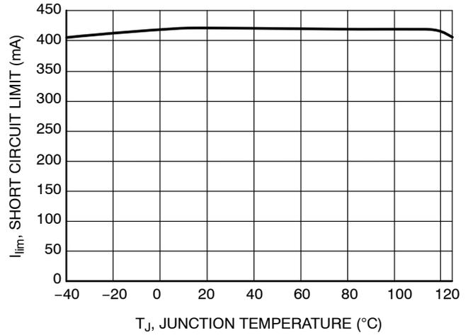
**Figure 8. Short Circuit Current Limit vs. Temperature for V<sub>out2</sub>**
