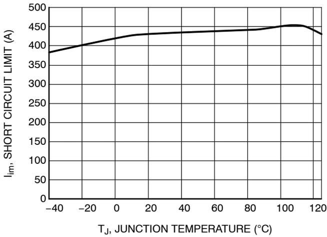
**Figure 7. Short Circuit Current Limit vs. Temperature for V<sub>out1</sub>**
