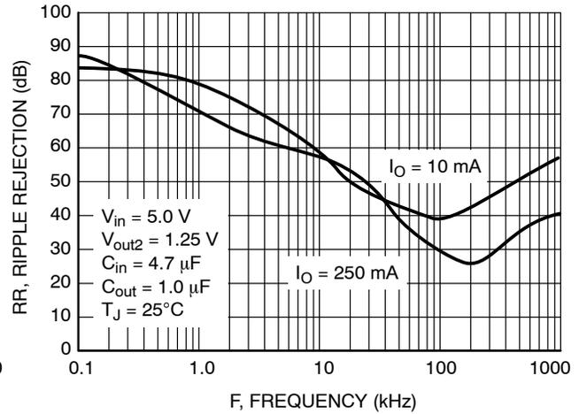
**Figure 10. Ripple Rejection vs. Frequency for V<sub>out2</sub>**
