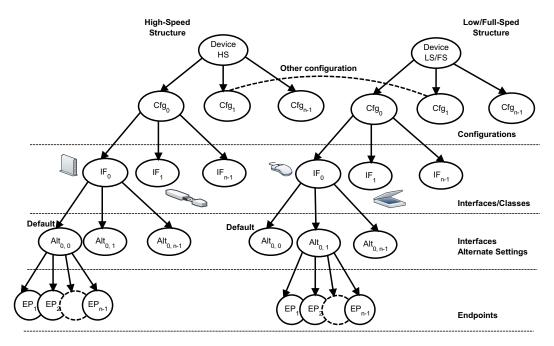
Figure 1-3 USB device structure
