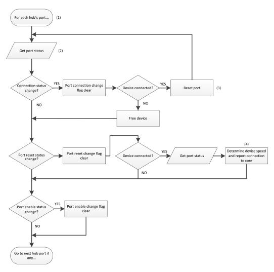
Figure 3-2 Hub Task State Machine
