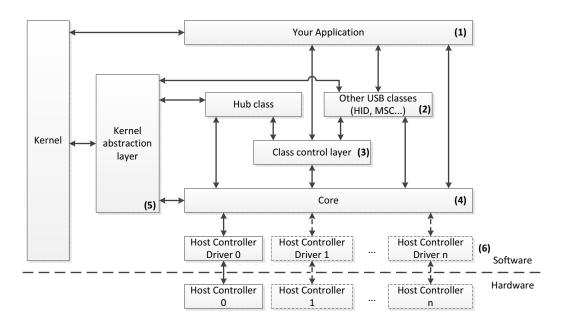
Figure 3-1 Overview of the  $\mu$ C/USB-Host Stack
