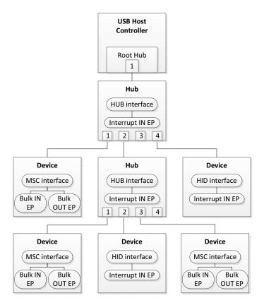
Figure 4-5 Single Host Controller and Multiple Devices Configuration
