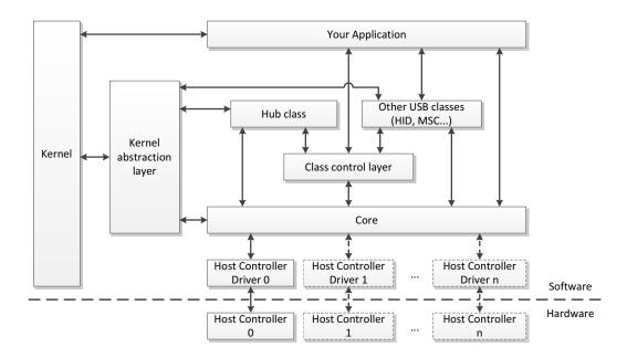
Figure 9-1  $\mu$ C/USB-Host Interactions with the Kernel
