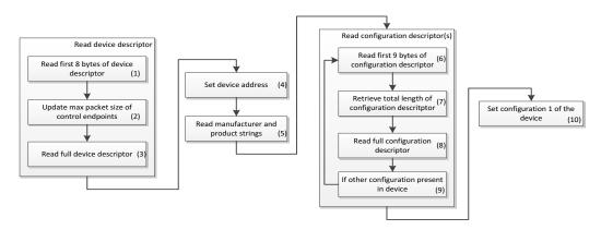
Figure 3-3 Enumeration Process as Executed by μC/USB-Host
