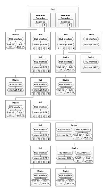
Figure 4-6 Multi-Host Controllers and Multiple Devices Configuration
