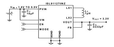
FIGURE 1. TYPICAL APPLICATION: VOLT = 3.3V
