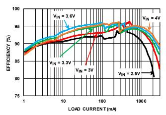
FIGURE 2. EFFICIENCY: V<sub>OUT</sub> = 3.3V
