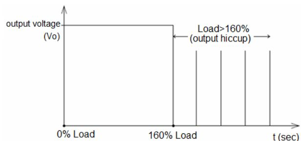
Additionally, if the 12 Volts' lout is  $>100\%$ ; but  $<160\%$  for a prolonged period of time (depending on the load), the Over Temperature Protection (OTP) will be activated due to high temperature on critical components. The power supply will then go into latch mode.
