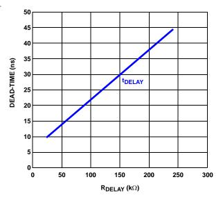
FIGURE 4. ADDITIONAL PROGRAMMED DEAD-TIME (t<sub>DELAY</sub>) vs DELAY RESISTOR VALUE
