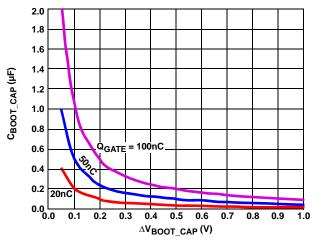
FIGURE 5. BOOTSTRAP CAPACITANCE vs BOOT RIPPLE VOLTAGE
