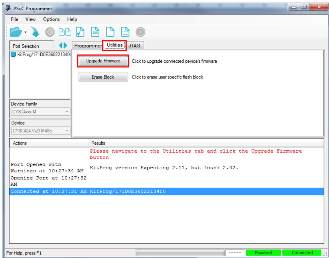
On successful upgrade, the Actions and Results window displays the firmware update message with the KitProg version, as shown in Figure 3-10.
