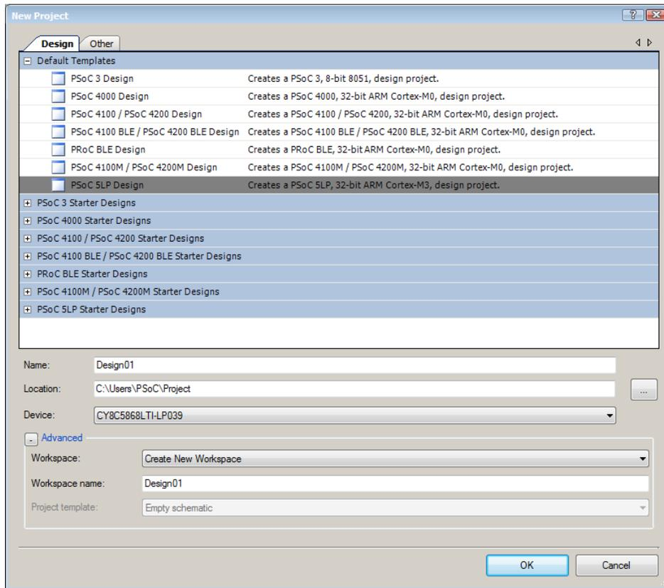
Figure 7-3. Select Device in PSoC Creator
