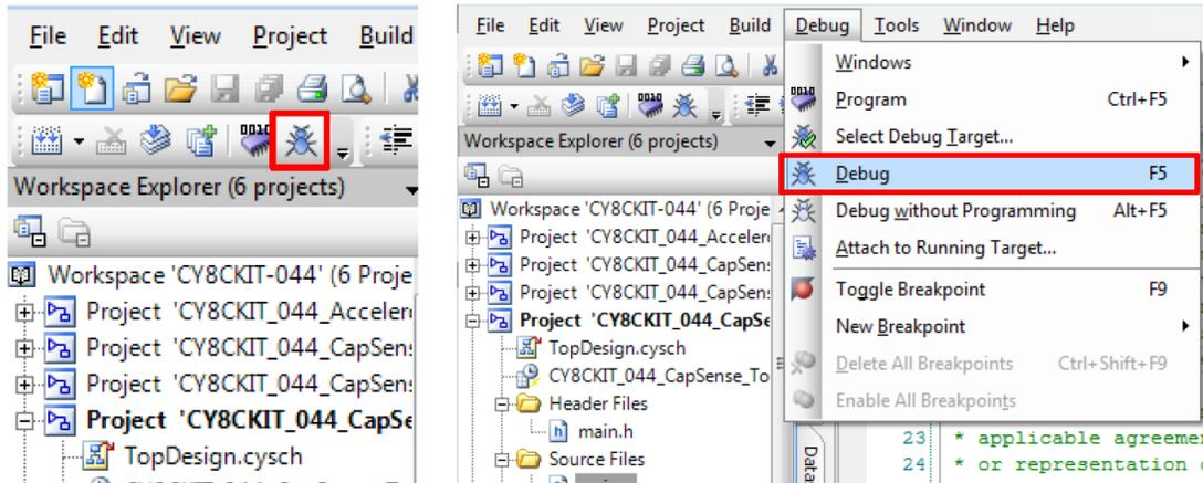
2. When PSoC Creator enters the Debug mode, use the buttons on the toolbar or keyboard shortcuts to debug your project.
