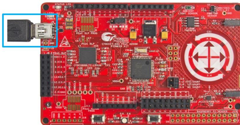
Figure 3-2. USB Male Connector J6 to PC USB Female Connector (Prototyping Kits)
