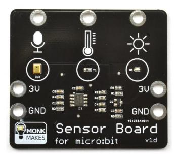
The MonkMakes Sensor Board for micro:bit allows you to sense sound level, temperature and light level.
