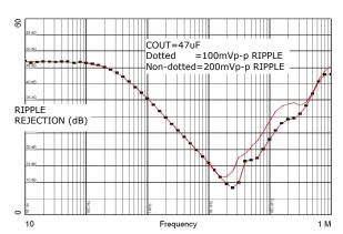
Fig. 13: PSRR, 50mA, 1.5VIN, 1VOUT, 47uF COUT
