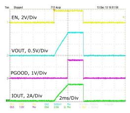
Fig. 12: Enable turn on/off, 3A, 1.5VIN, 1VOUT
