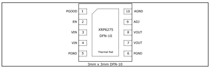
Fig. 3: XRP6275 Pin Assignment
