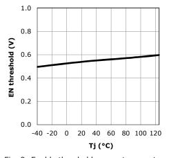
Fig. 9: Enable threshold versus temperature
