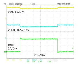
Fig. 14: Current limit, 1.5VIN, 1VOUT
