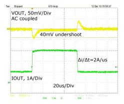
Fig. 7: Transient response, 1A-3A, 1.5VIN, 1VOUT
