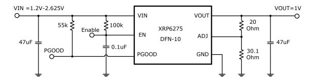
Fig. 15: XRP6274/5 Typical Application Diagram
