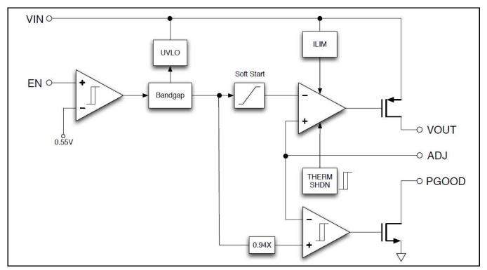
Fig. 2: XRP6275 Block Diagram
