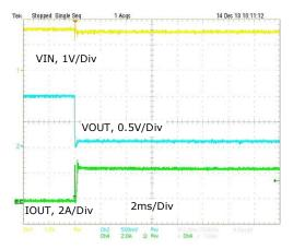
Fig. 5: Short-circuit, 1.5VIN, 1VOUT
