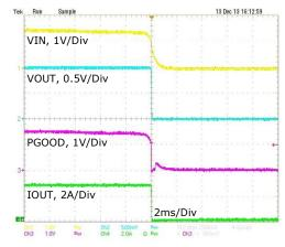
Fig. 11: Powerdown, IOUT=3A, 1.5VIN, 1VOUT
