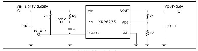
Fig. 1: XRP6275 Application Diagram
