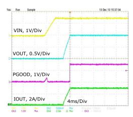
Fig. 10:Powerup, IOUT=3A, 1.5VIN, 1VOUT
