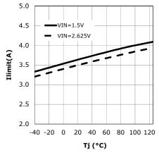
Fig. 8: Ilimit versus temperature
