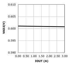
Fig. 4: VADJ versus IOUT, 1.5VIN, 1VOUT
