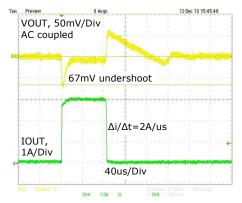
Fig. 6: Transient response, 20mA-3A, 1.5VIN, 1VOUT
