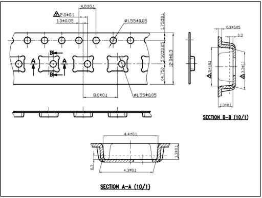
Figure 7: Carrier tape with microphone (top view)
