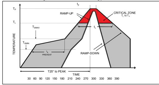
Figure 10: Recommended soldering profile limits
