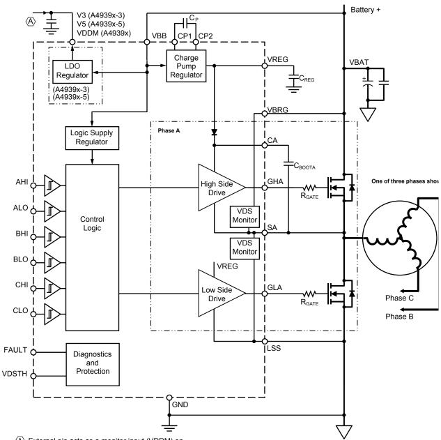
External pin acts as a monitor input (VDDM) on variants without LDO regulator, and a supply voltage output on variants with LDO regulator (designated V3 or V5 for 3.3 V and 5.0 V variants respectively)
