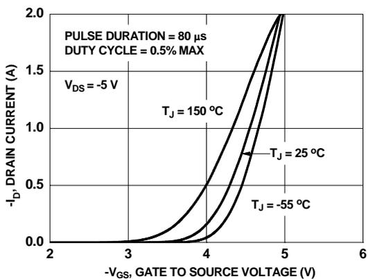
Figure 5. Transfer Characteristics
