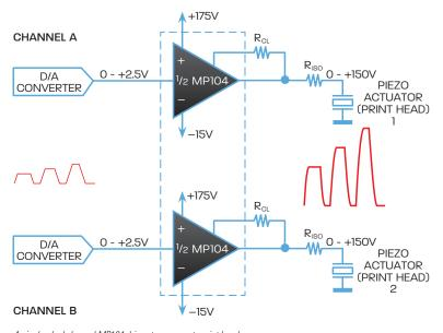
A single, dual channel MP104 drives two separate print heads.
