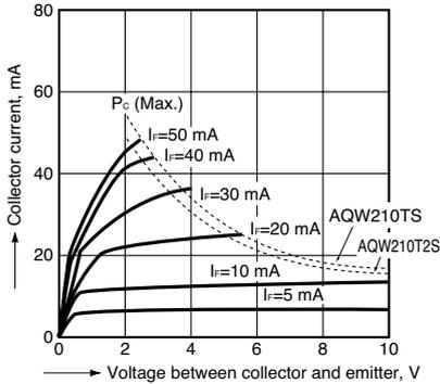
4-2. Collector current vs. voltage between collector and emitter characteristics ( $I_C$ - $V_{CE}$ )
