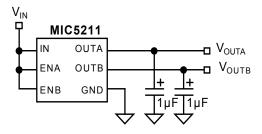
Figure 1. Thermal Conditions Circuit
