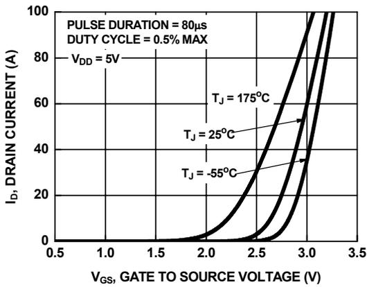
Figure 7. Transfer Characteristics
