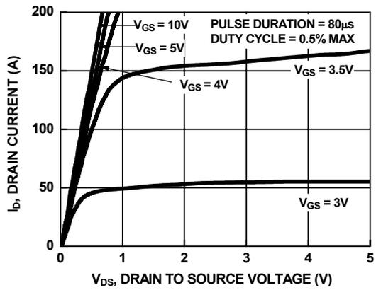
Figure 8. Saturation Characteristics
