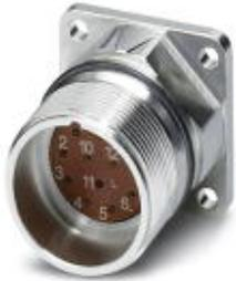
Device connector, front mounting, straight, Screw locking, M23, Number of positions: 12, Type of contact: Socket, Crimp connection, Axial O-ring, 4xØ3,2, Shielded: Yes
