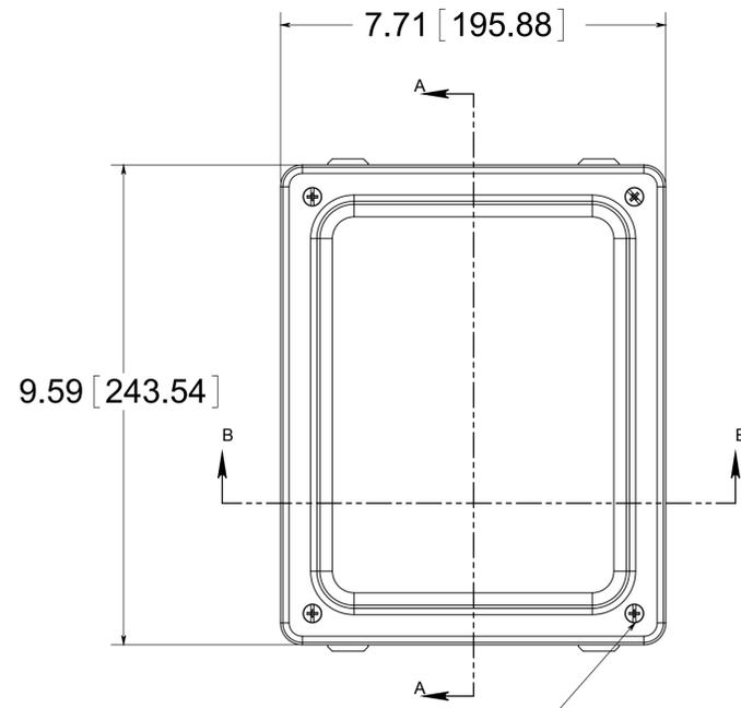
(4) EACH #10-32 BRASS INSERTS, AND STAINLESS STEEL CAPTIVE COVER SCREWS WITH RETAINING O-RING
