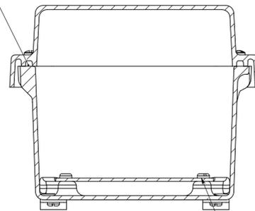
(4) EACH #10-32 BRASS INSERTS AND PLATED CARBON STEEL SCREWS
