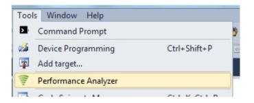
3. If not already preprogrammed - program the node with the Performance Analyzer FW available in the "Wireless Performance Analyzer Firmware extension" or from source code provided in ASF.
