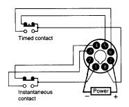
ON Motor and clutch (2-7)OFF ON NC (8-5) Time-limit ON contacts NO (8-6) ON NC (1-4) OFF Instantaneous ON NO (1-3) contacts OFF Timing operation indicator T = set time Rt = reset time
