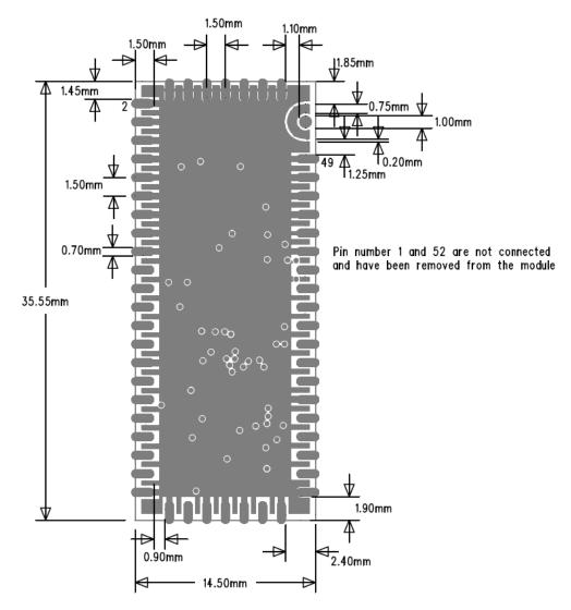
Figure 4: Physical dimensions (top view)
