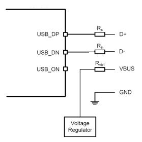
Figure 14: USB Connections for Bus-Powered Mode
