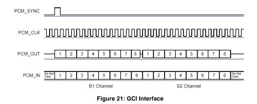
The start of frame is indicated by the rising edge of PCM\_SYNC and runs at 8kHz. With WT41-E in Slave mode, the frequency of PCM\_CLK can be up to 4.096MHz.
