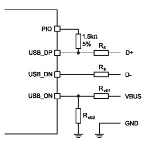
Figure 12: USB Connections for Self-Powered Mode
