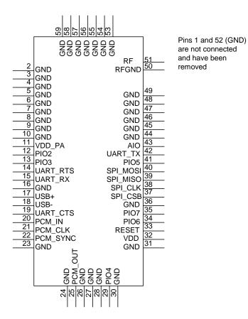
Figure 1: WT41-E pin out
