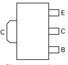
Pinout - top view
