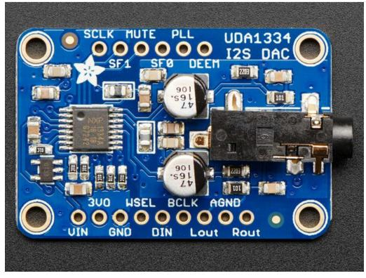
The UDA1334A is an **I2S** amplifier - it does not use analog inputs, it only has digital audio input support! Don't confuse I2S with I2C, I2S is a sound protocol whereas I2C is for small amounts of data.
