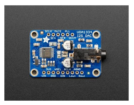
For inputs, you can use classic I2S (the default) or 16-bit, 20-bit or 24-bit left justified data. You can set it up to take an input system/master clock but we default-set it to just generate it for you, so you only need to connect Data In, Word Select (Left/Right Clock) and Bit Clock lines. If you want, there's a mute pin and a de-emphasis filter you can turn on.
