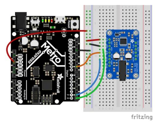
We can then run this demo which will generate a sine wave on both left and right channels. Try tweaking the sample rate, amplitude and frequency, see how the quality and volume changes!
