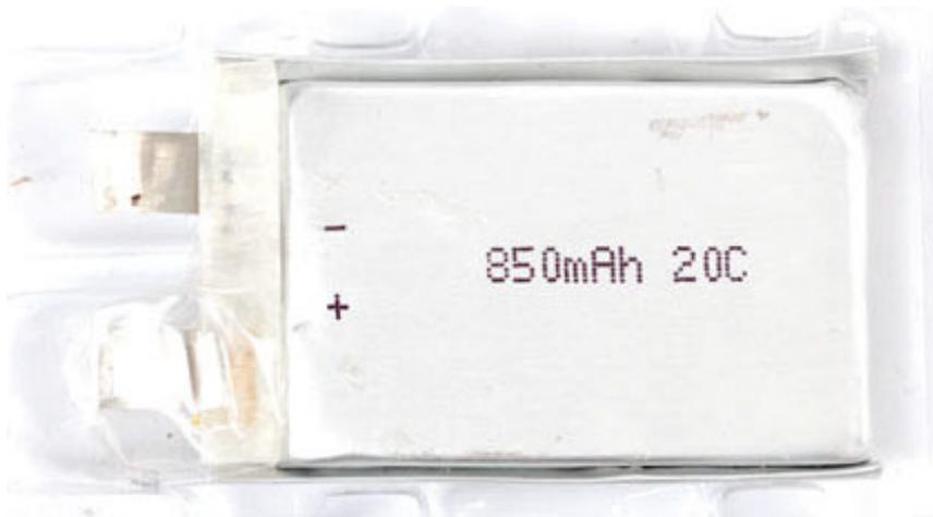
Important Note! Unless you are specifically building an RC device like a quadcopter, we suggest that you should never use RC lithium ion batteries for DIY projects. They do not have protection circuitry and are designed to not be safe. They have a much higher risk of exploding or catching on fire. If you need more current capability, just go with a larger lithium ion/polymer battery
