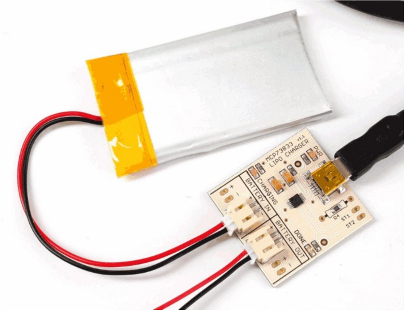
The **PWR** red LED on either board will light up to let you know its powered properly. While charging, an LED will also be lit. For the USB only charger, a green done LED will light when the battery is full. For the USB/DC charger, the charging LED will blink slowly (once every few seconds).
