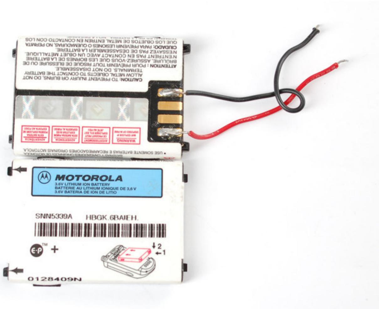
You may end up using camcorder or cell phone batteries. These are removable batteries in a hard case. They tend to have protection cells inside the case. This battery for example, is an old project battery from before you could buy li-poly batteries easily.
