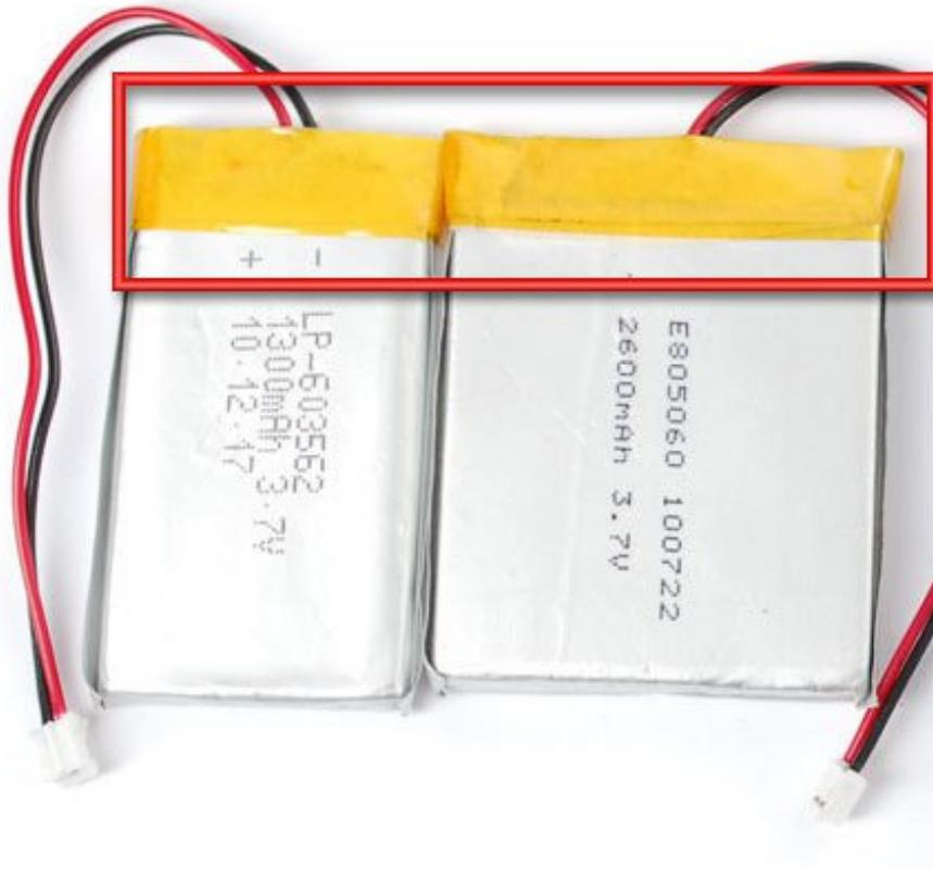
If you don't see any taped circuit board, the cell may be 'raw' - these raw cells **are not** protected!
