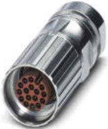
Cable connector, straight, Screw locking, M17, Number of positions: 8, Type of contact: Male connector, Crimp connection, shielded: yes, Cable diameter: 5 mm...8 mm
