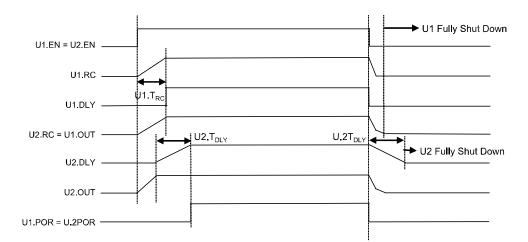
Tracking Dual Power Supply for I/O and Core Voltage of  $\mu Processor$
