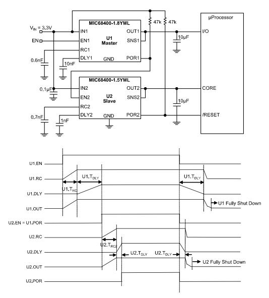
Sequenced Dual Power Supply for I/O and Core Voltage of µProcessor
