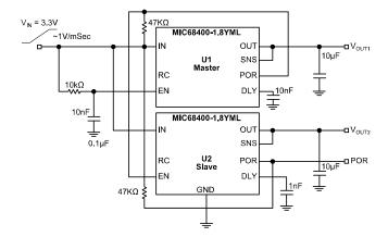
Enable Connection for V<sub>IN</sub>-Driven and/or Slow Rise-Time Inputs
