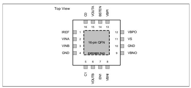
Figure 3 - 16-Pin QFN Diagram
