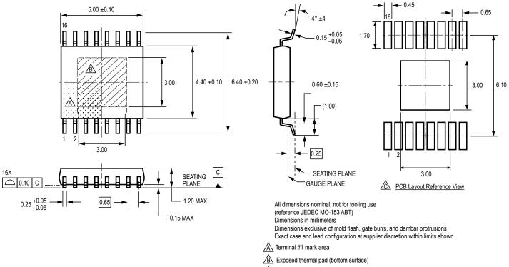
Reference land pattern layout (reference IPC7351 SOP65P640X110-17M); All pads a minimum of 0.20 mm from all adjacent pads; adjust as necessary to meet application process requirements and PCB layout tolerances; when mounting on a multilayer PCB, thermal vias at the exposed thermal pad land can improve thermal dissipation (reference EIA/JEDEC Standard JESD51-5)
