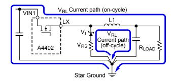
Figure 2. Current limiting during overload
