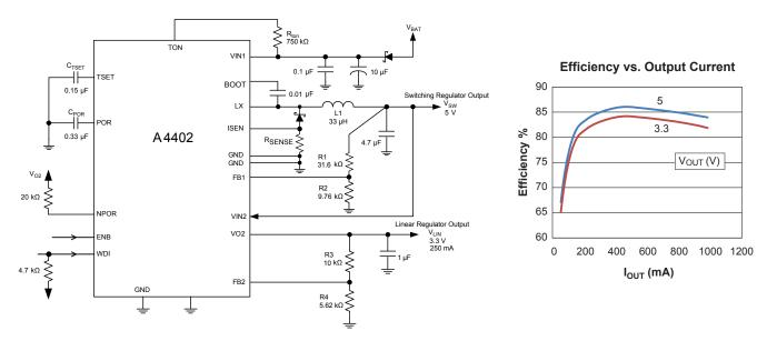
Data is for reference only. Efficiency data from circuit shown in left panel.
