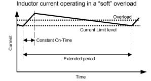
Figure 1. Current limiting during overload
