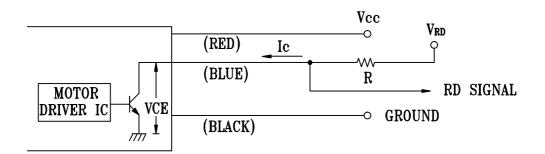
CAUTION: THE RD SIGNAL LEAD WIRE MUST BE KEPT AWAY FROM "+" LEAD WIRE & "-" LEAD WIRE.
