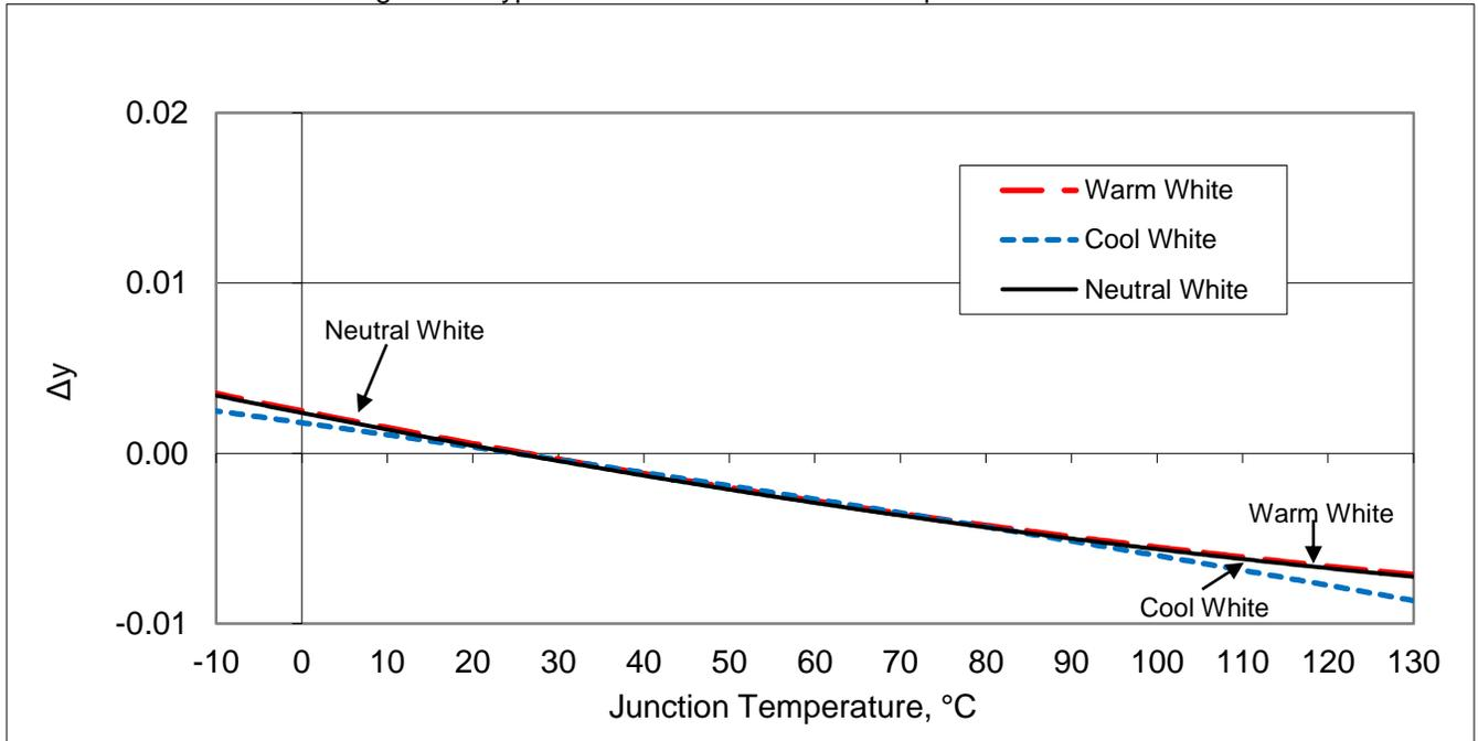
Figure 5: Typical ccy Shift vs. Junction Temperature
