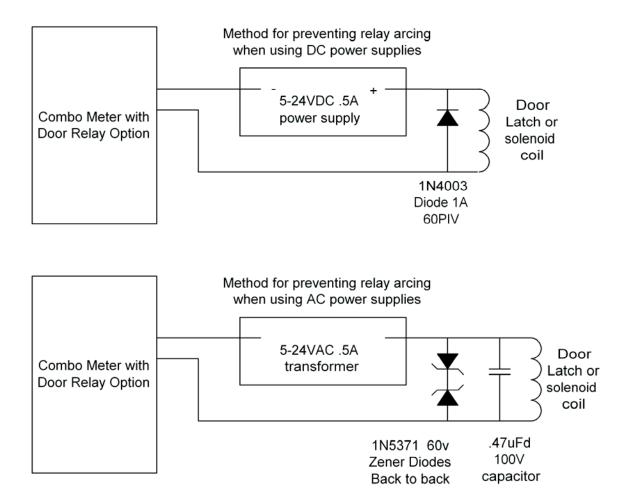
If the door relay contact is in series with a high current inductive load door latch such as a large solenoid or electromagnet, then arcing can develop across the relay contact when the contact breaks the circuit, and shorten the relay life.
