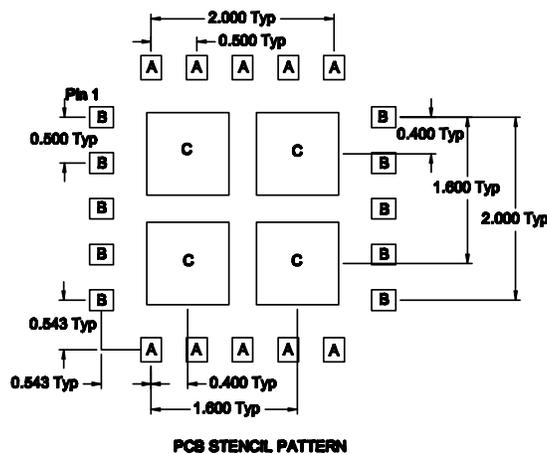
Thermal vias for center slug "C" should be incorporated into the PCB design. The number and size of thermal vias will depend on the application, the power dissipation, and this electrical requirements. Example of the number and size of vias can be found on the RFMD evaluation board layout.
