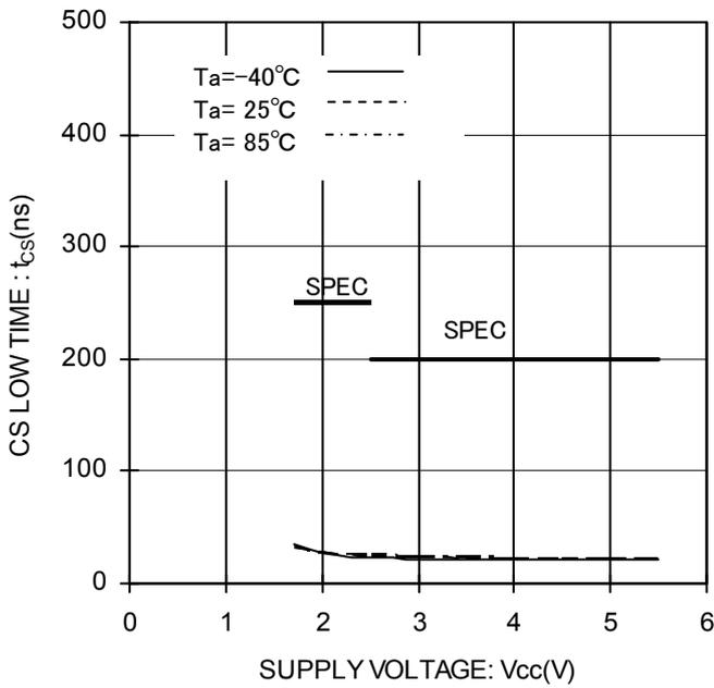
Figure 24. CS Low Time vs Supply Voltage
