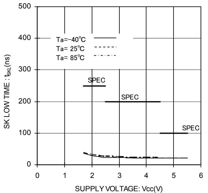
Figure 23. SK Low Time vs Supply Voltage
