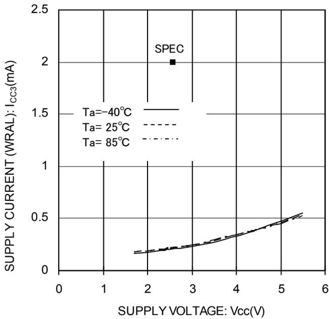
Figure 18. Supply Current (WRAL) vs Supply Voltage (f<sub>SK</sub>=1MHz)
