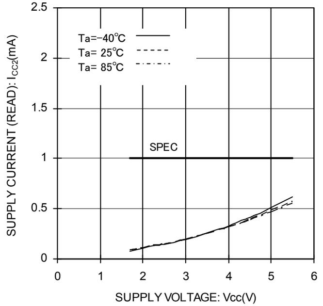
Figure 17. Supply Current (READ) vs Supply Voltage (f<sub>SK</sub>=3MHz)
