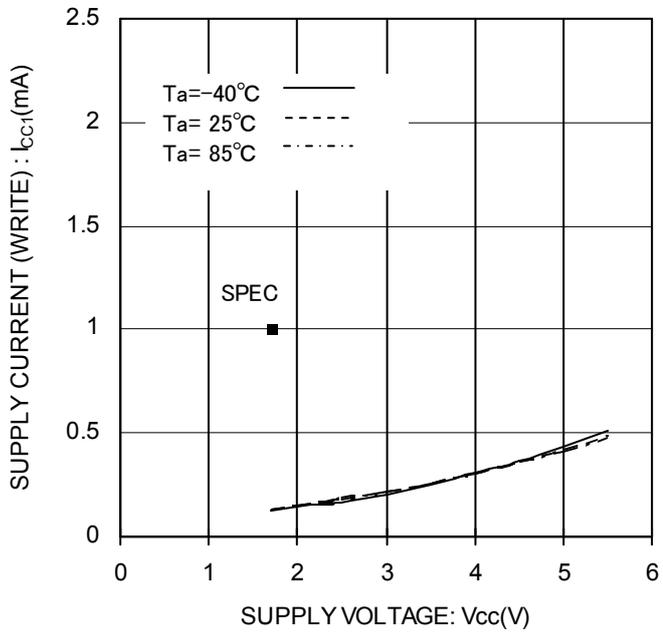
Figure 14. Supply Current (WRITE) vs Supply Voltage (f<sub>SK</sub>=1MHz)
