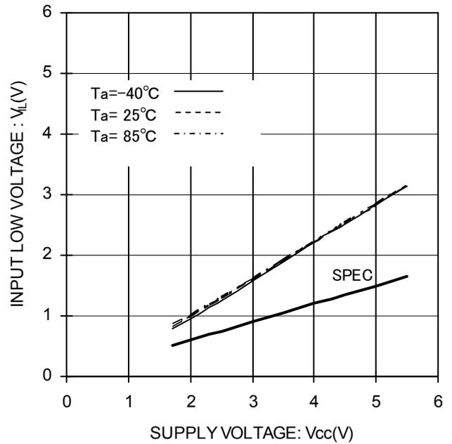
Figure 5. Input Low Voltage vs Supply Voltage (CS,SK,DI)
