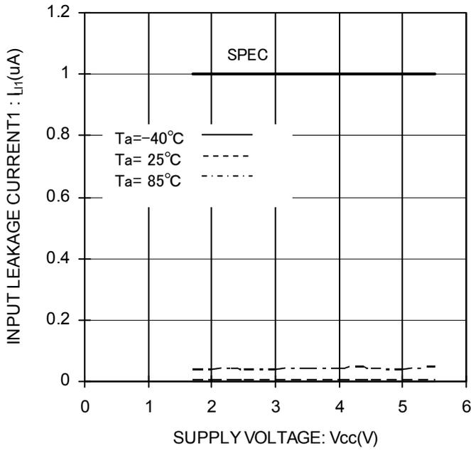
Figure 12. Input Leakage Current1 (DI) vs Supply Voltage
