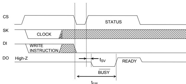
Figure 48.  $\overline{RDY}$ / $\overline{BUSY}$  STATUS Output Timing Chart
