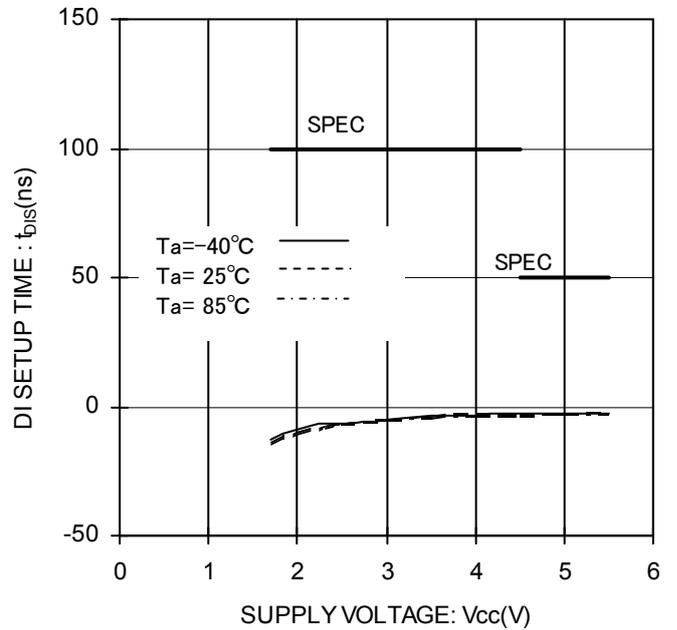
Figure 27. DI Setup Time vs Supply Voltage
