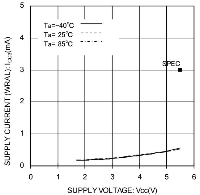
Figure 19. Supply Current (WRAL) vs Supply Voltage (f<sub>SK</sub>=3MHz)
