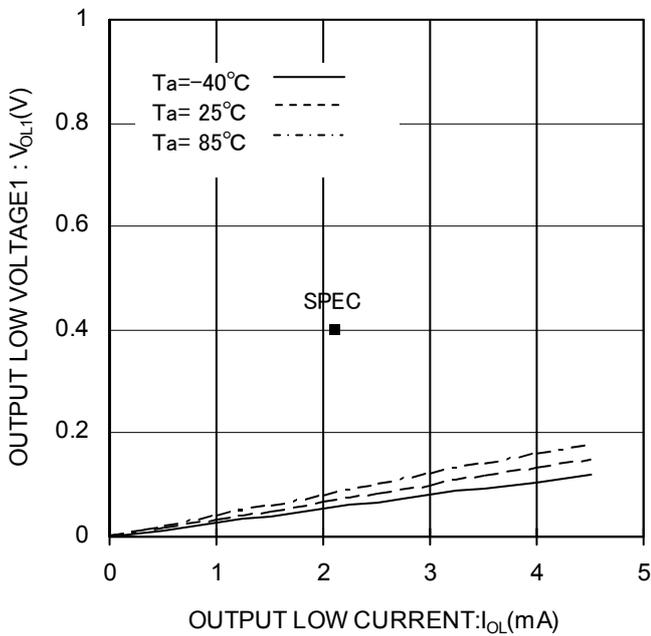
Figure 6. Output Low Voltage1 vs Output Low Current (V<sub>cc</sub>=2.7V)
