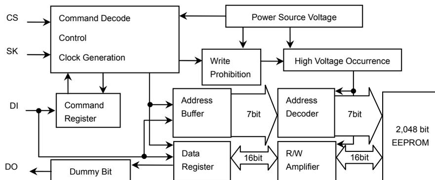
Figure 2. Block Diagram
