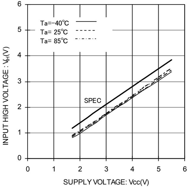
Figure 4. Input High Voltage vs Supply Voltage (CS,SK,DI)
