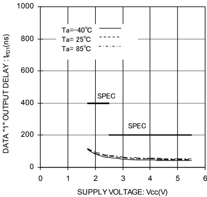
Figure 30. Data "1" Output Delay vs Supply Voltage
