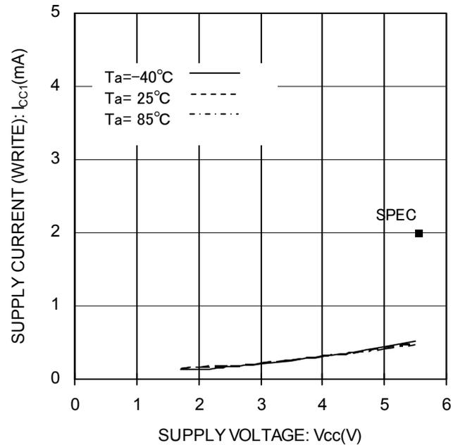
Figure 15. Supply Current (WRITE) vs Supply Voltage (f<sub>SK</sub>=3MHz)
