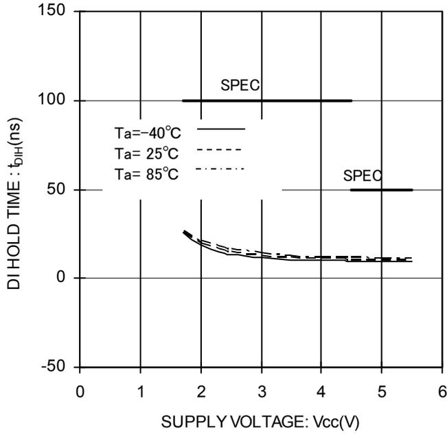
Figure 28. DI Hold Time vs Supply Voltage
