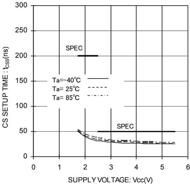
Figure 26. CS Setup Time vs Supply Voltage
