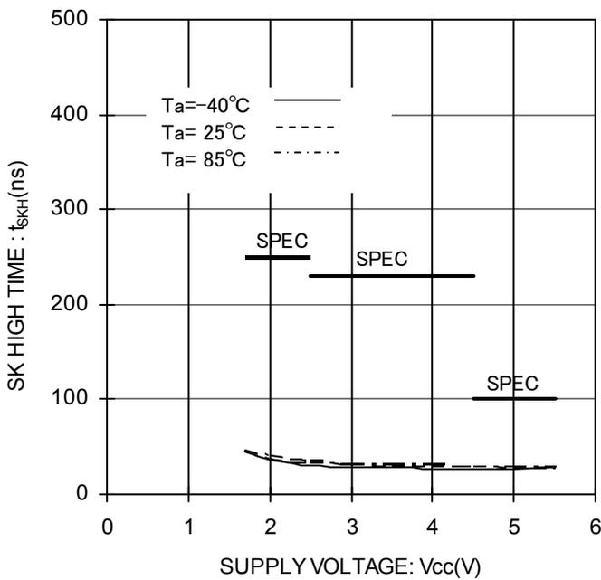
Figure 22. SK High Time vs Supply Voltage
