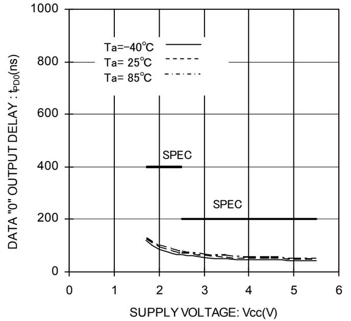
Figure 29. Data "0" Output Delay vs Supply Voltage
