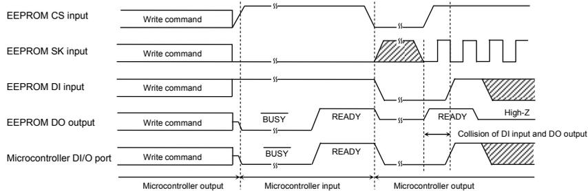
Figure 51. Collision Timing at DI, DO Direct Connection
