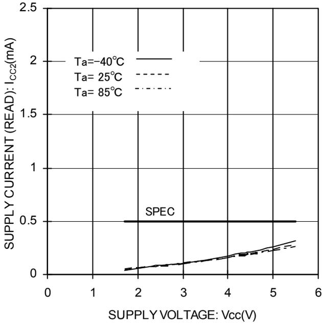
Figure 16 Supply Current (READ) vs Supply Voltage (f<sub>SK</sub>=1MHz)
