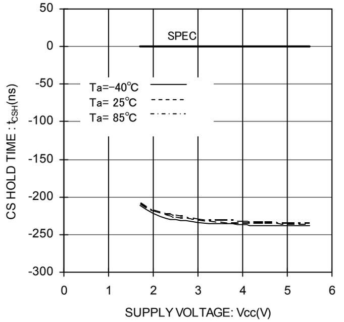
Figure 25. CS Hold Time vs Supply Voltage
