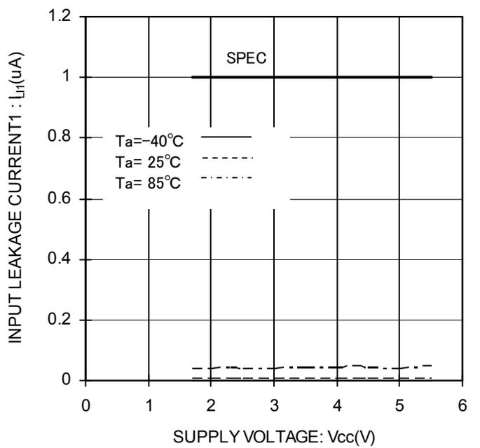
Figure 11. Input Leakage Current1 (SK) vs Supply Voltage
