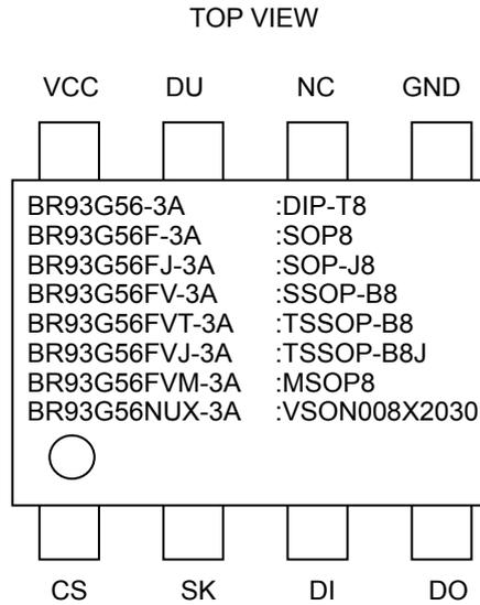
Figure 3. Pin Configuration
