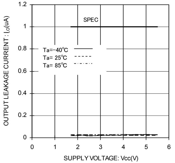
Figure 13. Output Leakage Current (DO) vs Supply Voltage
