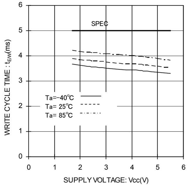
Figure 33. Write Cycle Time vs Supply Voltage
