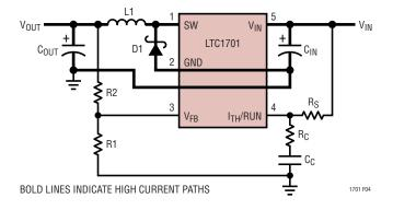
Figure 4. LTC1701 Layout Diagram (See Board Layout Checklist)
