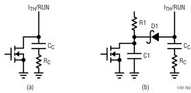
Figure 3. I<sub>TH</sub>/RUN Pin Interfacing
