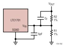
Figure 2. Setting the Output Voltage
