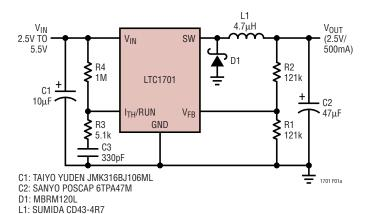
Figure 1. 2.5V/500mA Step-Down Regulator
