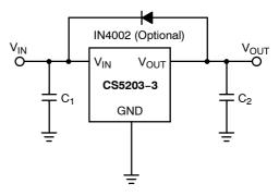
Figure 9. Protection Diode Scheme for Large Output Capacitors
