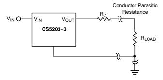
Figure 10. Conductor Parasitic Resistance Effects
