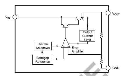
Figure 2. Block Diagram
