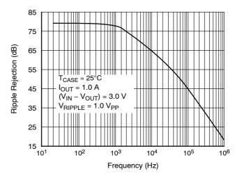
Figure 6. Ripple Rejection vs. Frequency
