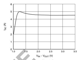
Figure 8. Short Circuit Current vs.  $V_{\text{IN}} - V_{\text{OUT}}$
