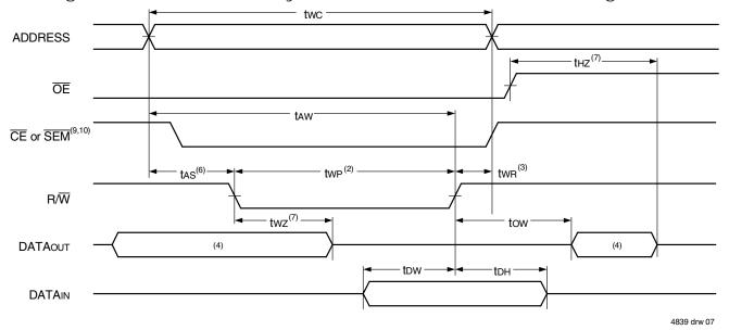
Timing Waveform of Write Cycle No. 2, **CE** Controlled Timing<sup>(1,5)</sup>
