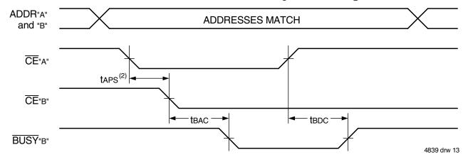
Waveform of **BUSY** Arbitration Cycle Controlled by Address Match Timing  $(M/S = VIH)^{(1)}$
