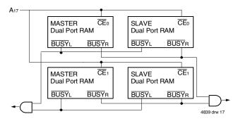
Figure 3. Busy and chip enable routing for both width and depth expansion with IDT7009 RAMs.
