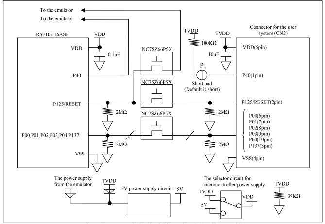
Figure 3 Internal circuit of this product (R0E510YLVB00)
