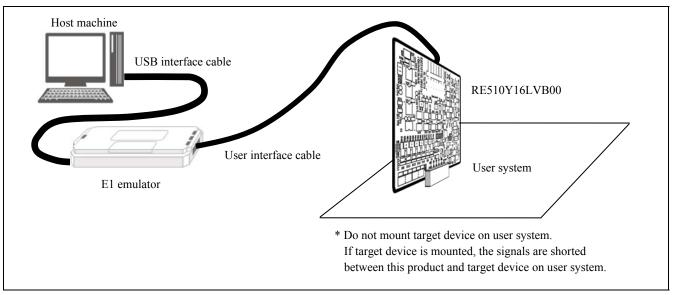
Figure 1 System Configuration
