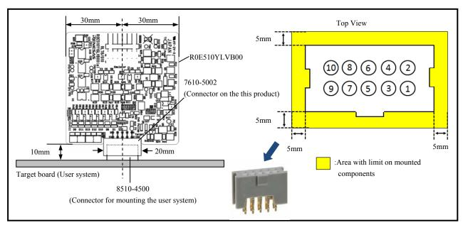
Figure 4 The connector for mounting user system and mounting connector
