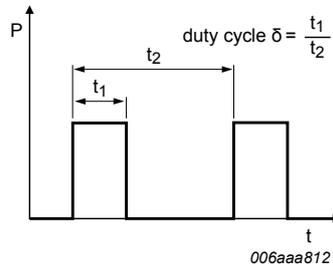
Fig. 17. Duty cycle definition
