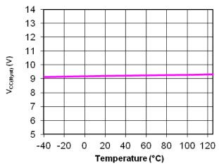
Figure 12. V<sub>CC(Hyst)</sub> vs. Junction Temperature
