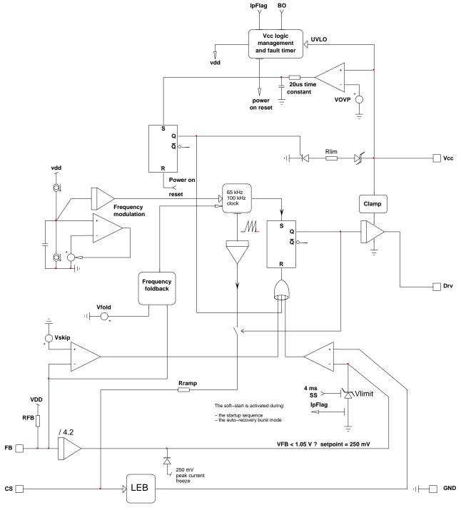
**Figure 2. Internal Circuit Architecture**
