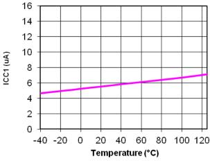
Figure 6. ICC1 vs. Junction Temperature
