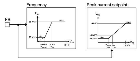
Figure 27. By Observing the Voltage on the Feedback Pin, the Controller Reduces its Switching Frequency for an Improved Performance at Light Load
