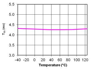
Figure 16.  $T_{SS}$  vs. Junction Temperature
