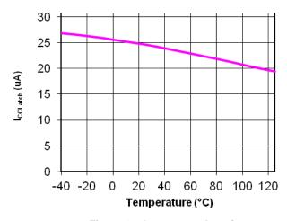
Figure 13. I<sub>CCLatch</sub> vs. Junction Temperature
