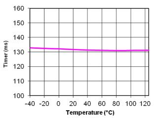
Figure 23. Timer vs. Junction Temperature
