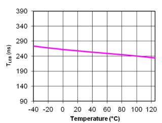
Figure 14. T<sub>LEB</sub> vs. Junction Temperature
