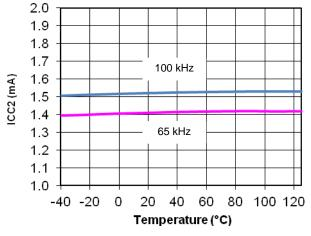
Figure 7. ICC2 vs. Junction Temperature
