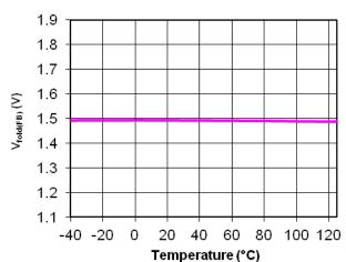
Figure 18. V<sub>fold(FB)</sub> vs. Junction Temperature
