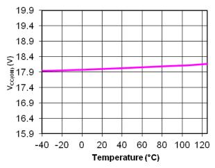
Figure 10. V<sub>CC(ON)</sub> vs. Junction Temperature
