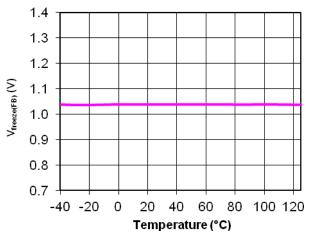
Figure 22. V<sub>freeze(FB)</sub> vs. Junction Temperature
