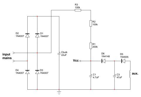
Figure 25. The Startup Resistor Can Be Connected to the Input Mains for Further Power Dissipation Reduction
