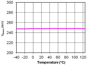
Figure 21. V<sub>freeze</sub> vs. Junction Temperature
