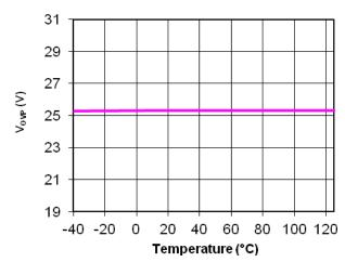
Figure 24. V<sub>OVP</sub> vs. Junction Temperature
