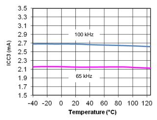
Figure 8. ICC3 vs. Junction Temperature
