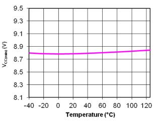
Figure 11. V<sub>CC(min)</sub> vs. Junction Temperature
