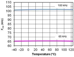
Figure 4. Fosc vs. Junction Temperature
