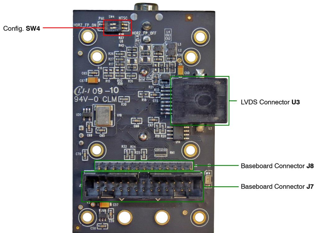
Figure 4. Bottom View of the Evaluation Board – Connector
