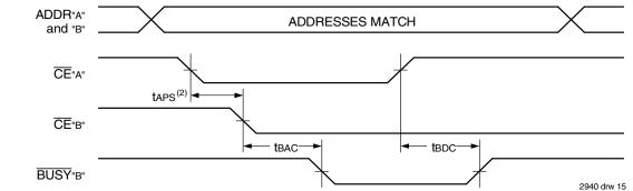
Waveform of **BUSY** Arbitration Cycle Controlled by Address Match Timing<sup>(1)</sup> (M/ $\mathbf{S}$  = VIH)
