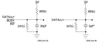
Figure 1. AC Output Test Load
