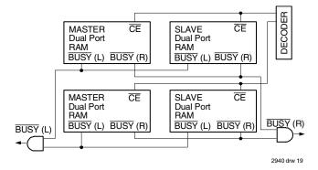
Figure 3. Busy and chip enable routing for both width and depth expansion with IDT7007 RAMs.
