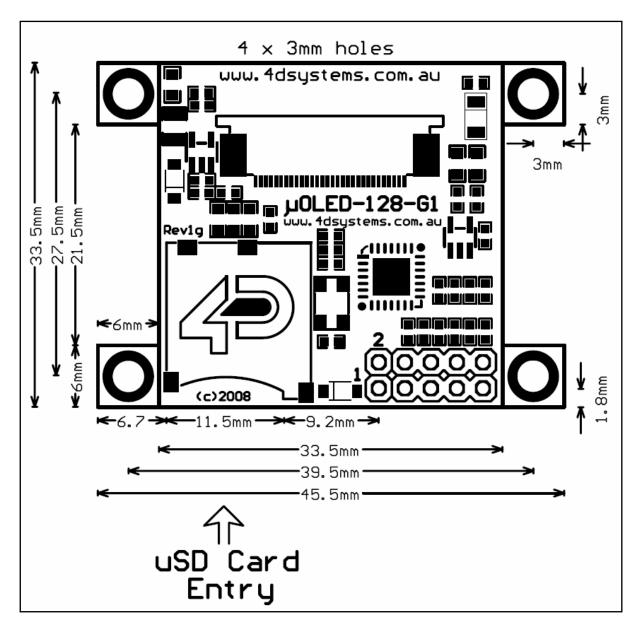
The module thickness is **6.3mm** (not including header pins)
