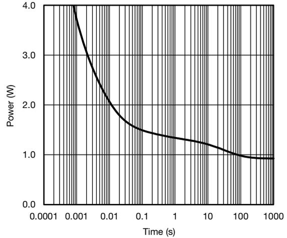
Single Pulse Power, Junction-to-Ambient <sup>a</sup>
