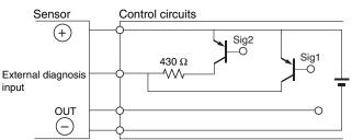
Note: Use a transistor that is capable of switching 50 mA at 10 V. The resistor must have a power rating of 1/8 W min.
